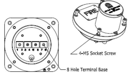
**CAUTION:** Before removing the cover, ensure the power to the product is isolated. Remove the four pieces of M5
